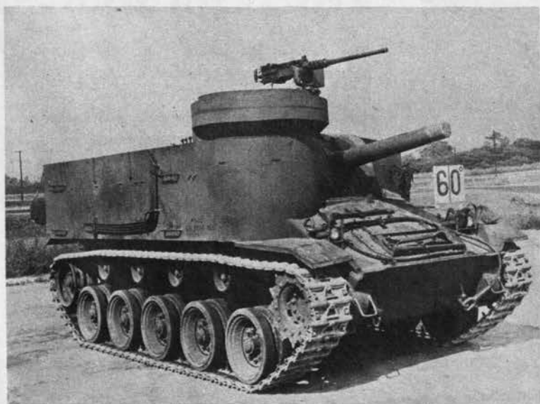
New Priest, M-37, has 105-mm. howitzer and superstructure similar to the M-7. M-24's torsion-bar suspension is chief recognitional change.
